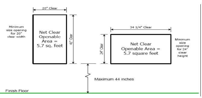
Minimum Net Clear Width/Height Requirements for Emergency Escape & Rescue Openings (Inches)
