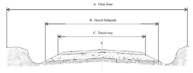
Figure A1 - Typical Roadway Cross Section
