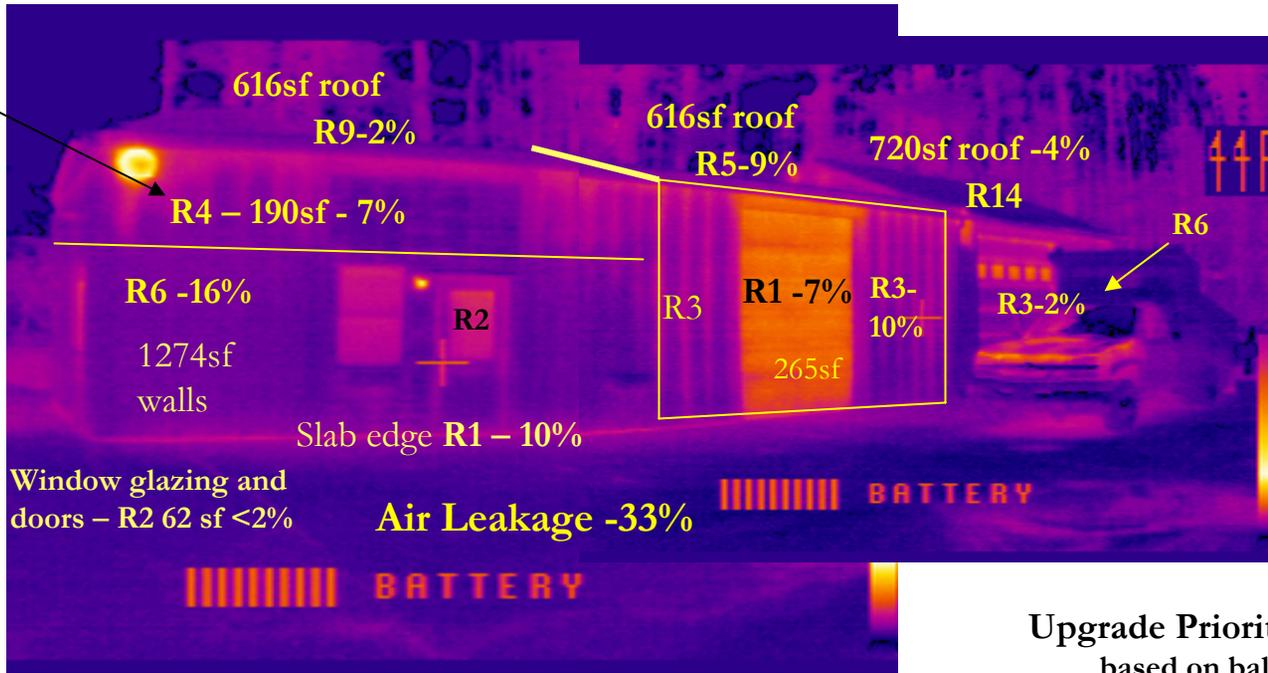
Brighter colors indicate heat greater rates of heat loss. Note most significant areas are middle door and walls, above the ceiling, slab edges, end garage door, and windows.
