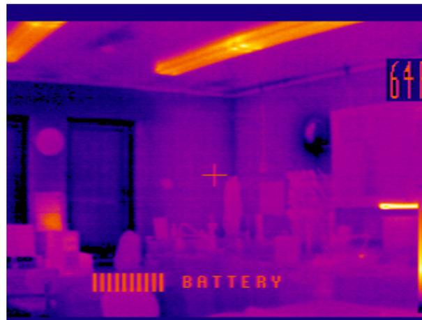
Window glazing accounts for less than 6% of the entire wall surface area from 6 casement windows and glass entry. The expense of replacement would take a long time to recover. However comprehensive air sealing would be a cost effective improvement.
