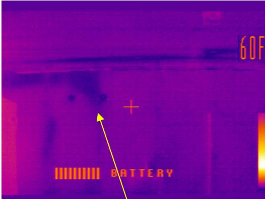
Batts settled and perimeter voids and air infiltration. Metal door needed to limit vandal damage. Building could be retrofitted to high performing, super insulated shed for between \$3-\$4K.
