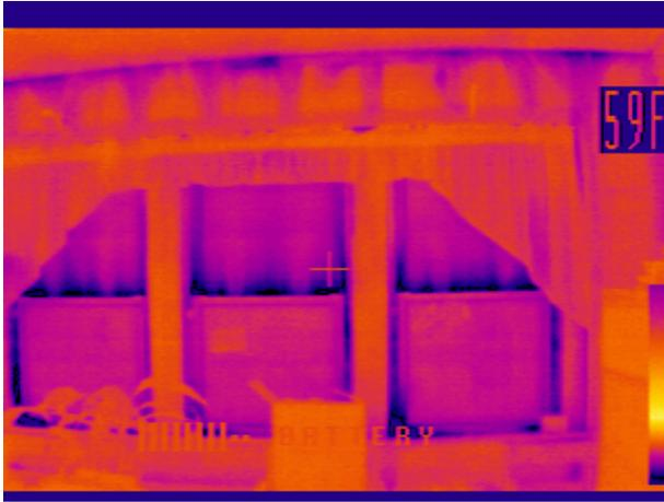
These images were taken with the blower door fan running and the building depressurized to -25 pascals. So while this is not a normal condition, it does approximate the kind of infiltration one could expect on a cold or windy day.
