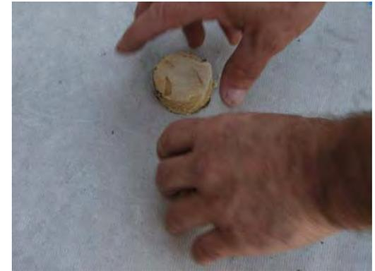
In 2009, a new stove hood exhaust was installed, and Victor Johnson did that as well. Victor kindly performed a core to verify insulation thickness (7/25/10). We found two layers of foil-faced polyiso – 1" over 2" for a total of 3". Aged performance slightly under R6 for a total R17+ on both roofs.
