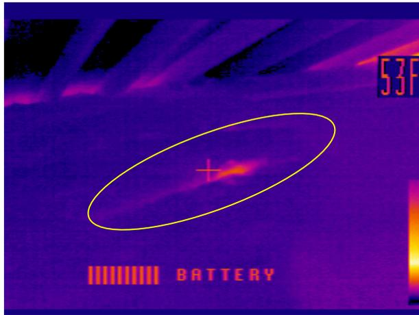
The end wall, shared with the garage, shows significant heat loss from the garage into this cold attic.
