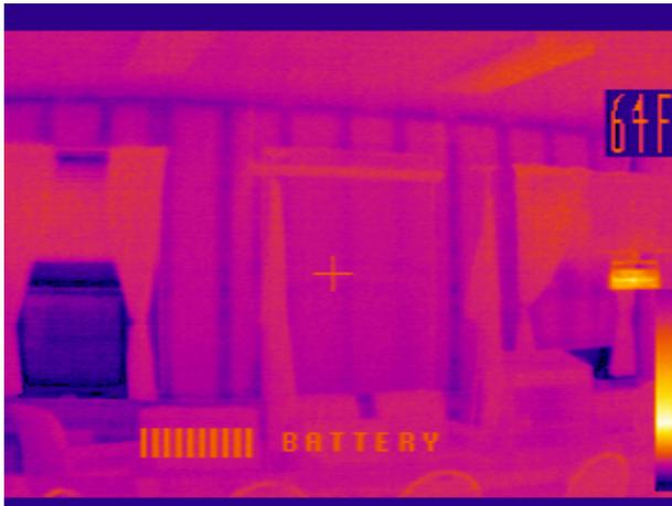
Conventional stud framing at 16"OC with insulated cavities and thermal bridging (greater rate of heat loss) at each stud.
