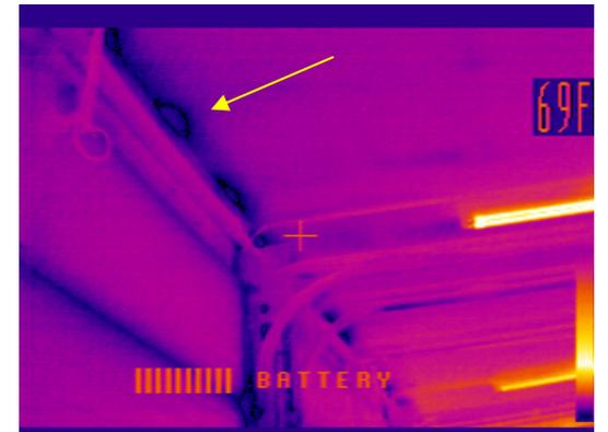
The garage ceiling has less air infiltration into the space, though there is still air movement evident between the joists and the drywall ceiling. Note the discoloring under joists as warmer, moist air condenses on the cooler surface below the wood joists. Unsealed / un-insulated top plates are typically colder and a source of air movement.
