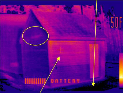
Solar radiation. Lower half of wall is cooler because there had been a sheet of plywood leaning on the wall – which was laid flat just before the picture.
