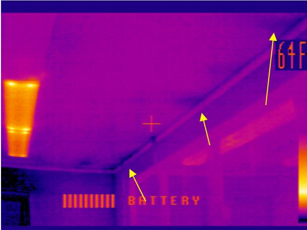
Cooling above the top plates is common, and often from air leakage ('wind washing') from soffits.
