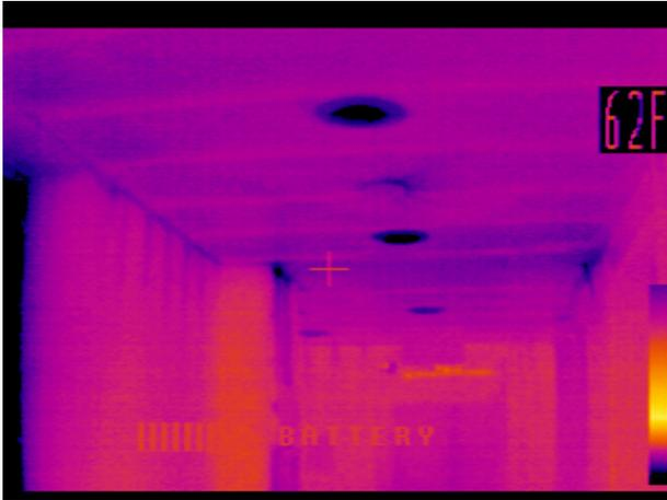
Slightly more pronounced heat loss under pressure. Note in both cases the rafters are warmer than the cavities, indicating low levels of effective insulation.
