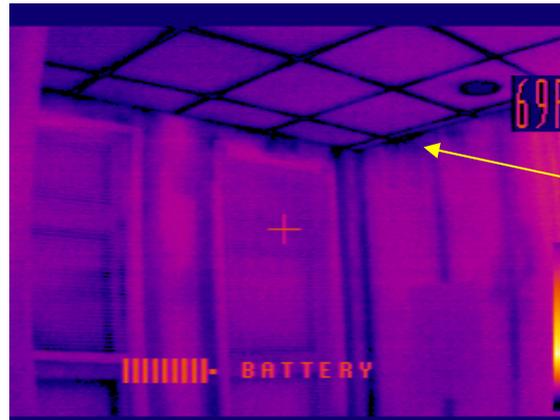
Cold, attic air being drawn down near the top plates and onto perimeter walls.
