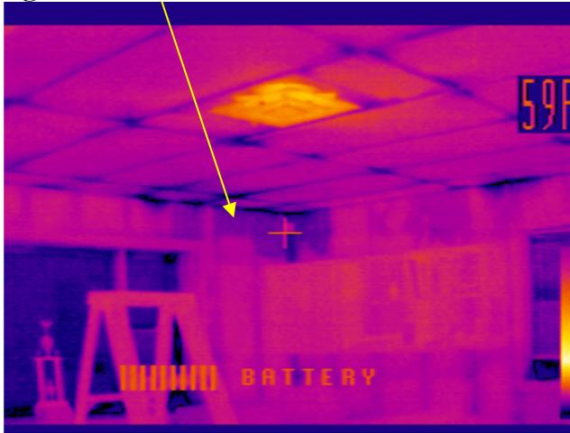
Gaps in air barrier create convective heat losses, as well as diminish R-value performance of existing insulation.
