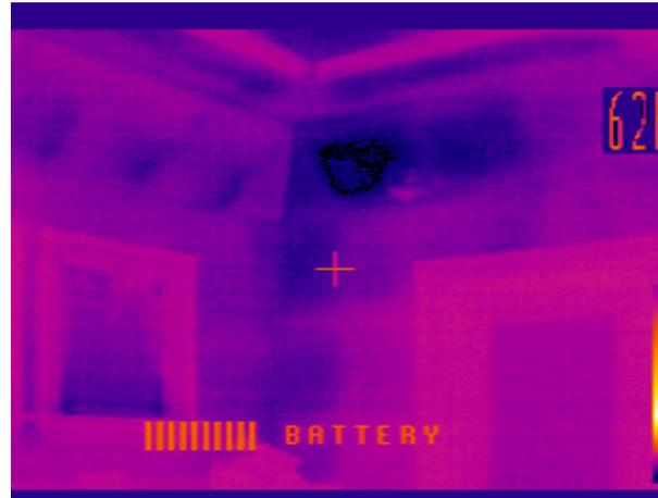
Blown and batt fiberglass insulation can be seen in the attic, however the raised dais over this vaulted ceiling area appears to be minimally insulated, especially at the sloped perimeter. There does not appear to be a continuous air barrier. Insulation levels and effectiveness can only be roughly gestimated.
