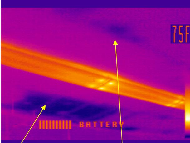
These cavity areas are completely void of insulation.
