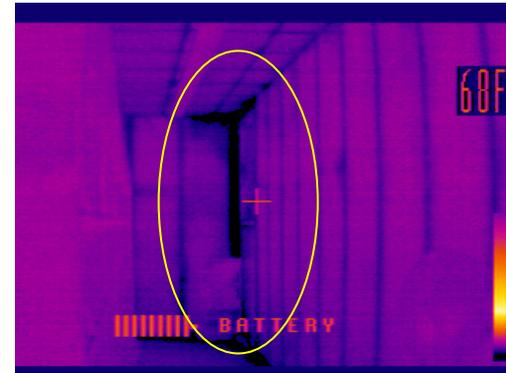
The fan below runs in the winter in an attempt to send heat to that cold corner. It is partly due to distribution issues, but far more to the air infiltration from the attic above and multiple metal studs in the corner.
