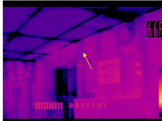
Note diminished insulating performance throughout walls where air (and moisture) are allowed to flow.
