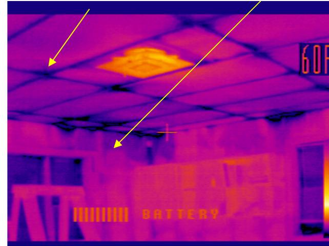
Inside temperature was 68°F and outside 39°F. IR image above on left was taken under normal conditions and the one on the left with the blower door fan running and the building depressurized to -30pascals with respect to outside.
