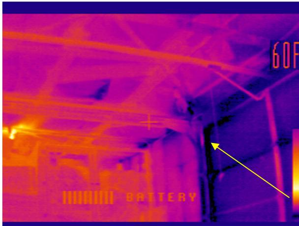
Note the reduced insulation value as the fiberglass is compressed. Darker color shades indicate greater heat loss.
