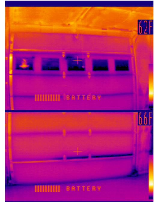
With or without the blower door fan running, air leakage around all doors edges, and trim, is significant.
