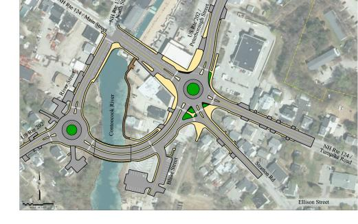
In addition to the proposed improvements to traffic flow through the five-leg intersection and along Route 202, the proposed improvements include new accommodations for pedestrians. The proposed connector roadway and bridge crossing the Contoocook River would provide sidewalk and a shoulder/bike lane on each side of the roadway.
