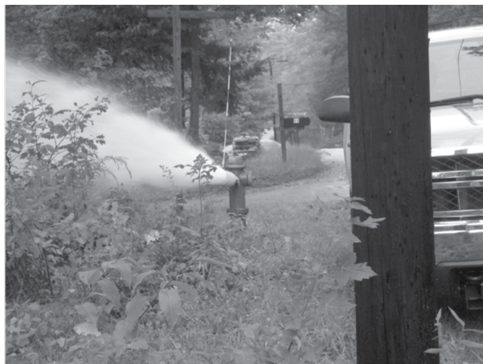
Hydrant flow testing performed in order to calibrate water distribution system model
