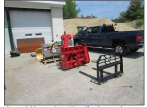
New Multi-Purpose Tractor with assorted attachments for roadside mowing, sidewalk winter maintenance and fork lift
