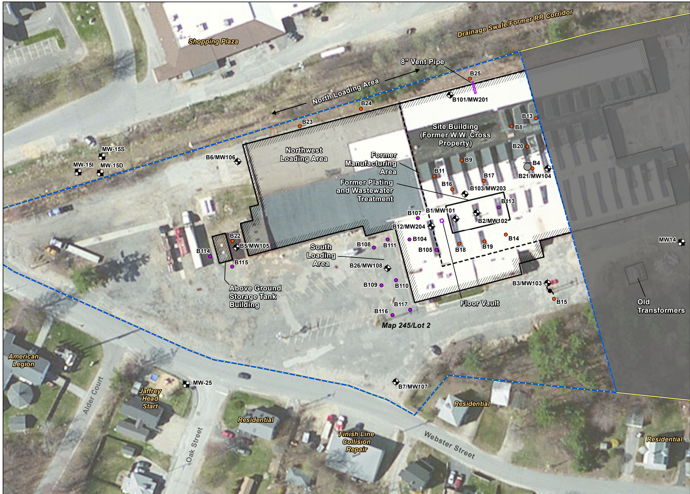
Figure 3 Boring/Monitoring Well Locations
